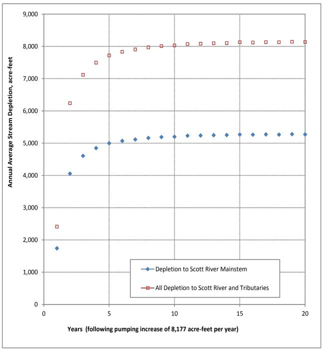
Note: The net increase in pumping is simulated as occurring as a single step; the resulting depletion curve can be used to identify lagged depletion impacts from a gradual change in pumping.
