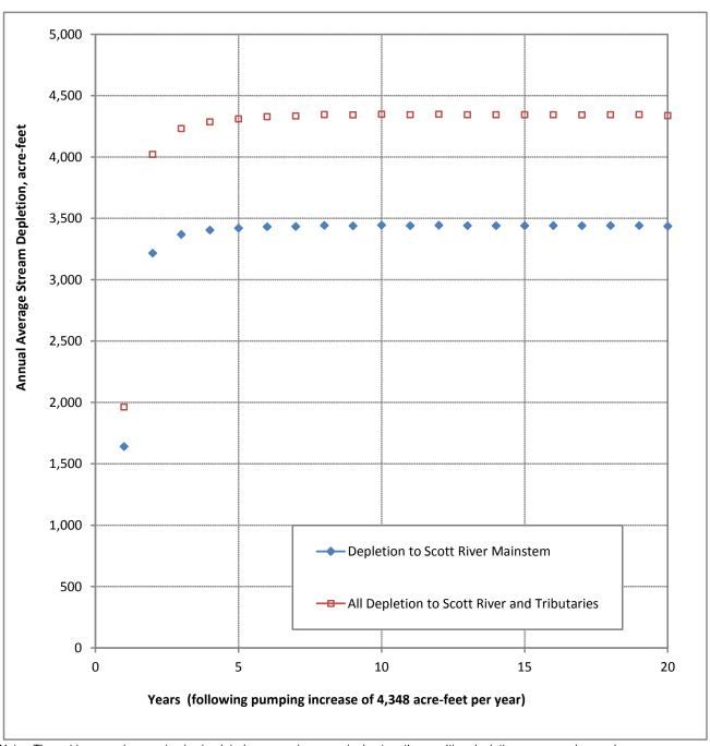
Note: The net increase in pumping is simulated as occurring as a single step; the resulting depletion curve can be used to identify lagged depletion impacts from a gradual change in pumping.
