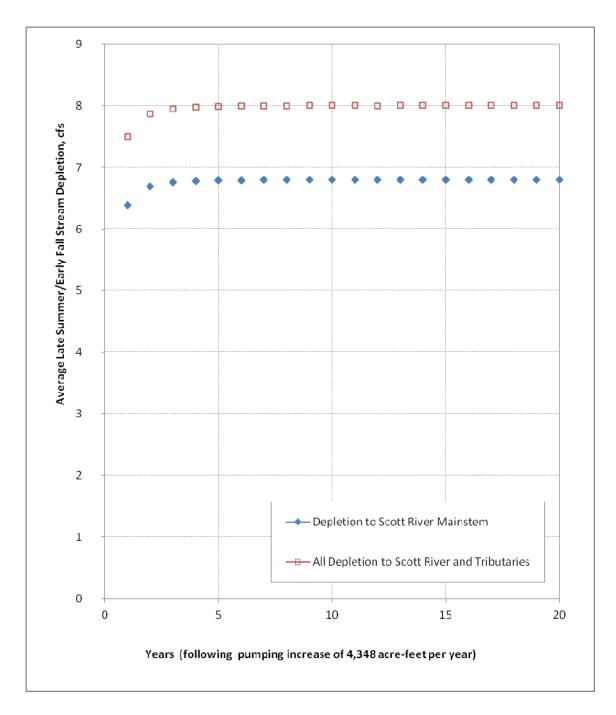
Note: The net increase in pumping is simulated as occurring as a single step; the resulting depletion curve can be used to identify lagged depletion impacts from a gradual change in pumping
